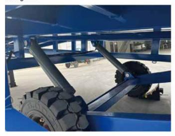
10. Place the manual outrigger in a vertical state, crank it until it touches the ground and fix it, and then fix the pivot pin.
