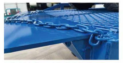
7. Steel chains-the ramp is fixed to the truck for safe operation
