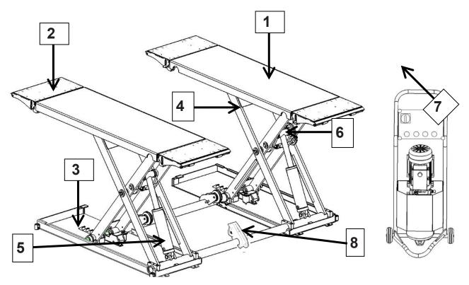
platforms (1) each equipped with N.2 ramps (2) which can be locked as the platform extensions, placed on the ground by means of base frames (3).
