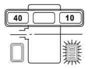
III Slowly turn the tire so that the outer indicator lights are all on. Put a 10g lead block just above the outer rim, as shown in the figure:
