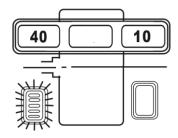
II Slowly turn the tire, when the inside lights are all on, put a 40g lead block on the inside side of the rim just above the vertical spindle, as shown in the figure:
