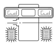
IV Press Start button to START. After braking, the display window shows 00. After balancing, remove the tire. If it does not reach 00, follow the steps above
