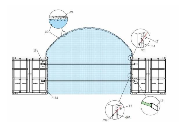
Assembly the cover according to above drawing.
