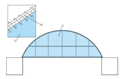
Assembly the frame first according to above drawing. Then use ropes No.8 to tie the cover to the frame.
