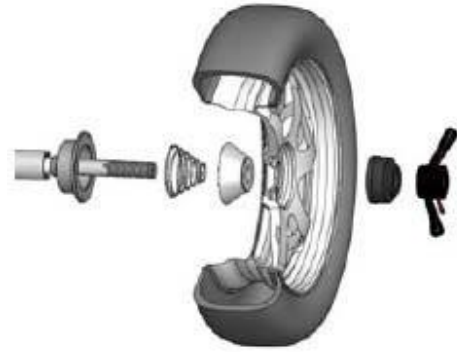
Main shaft → lower spring → suitable cone wheel → bowl → quick nut
