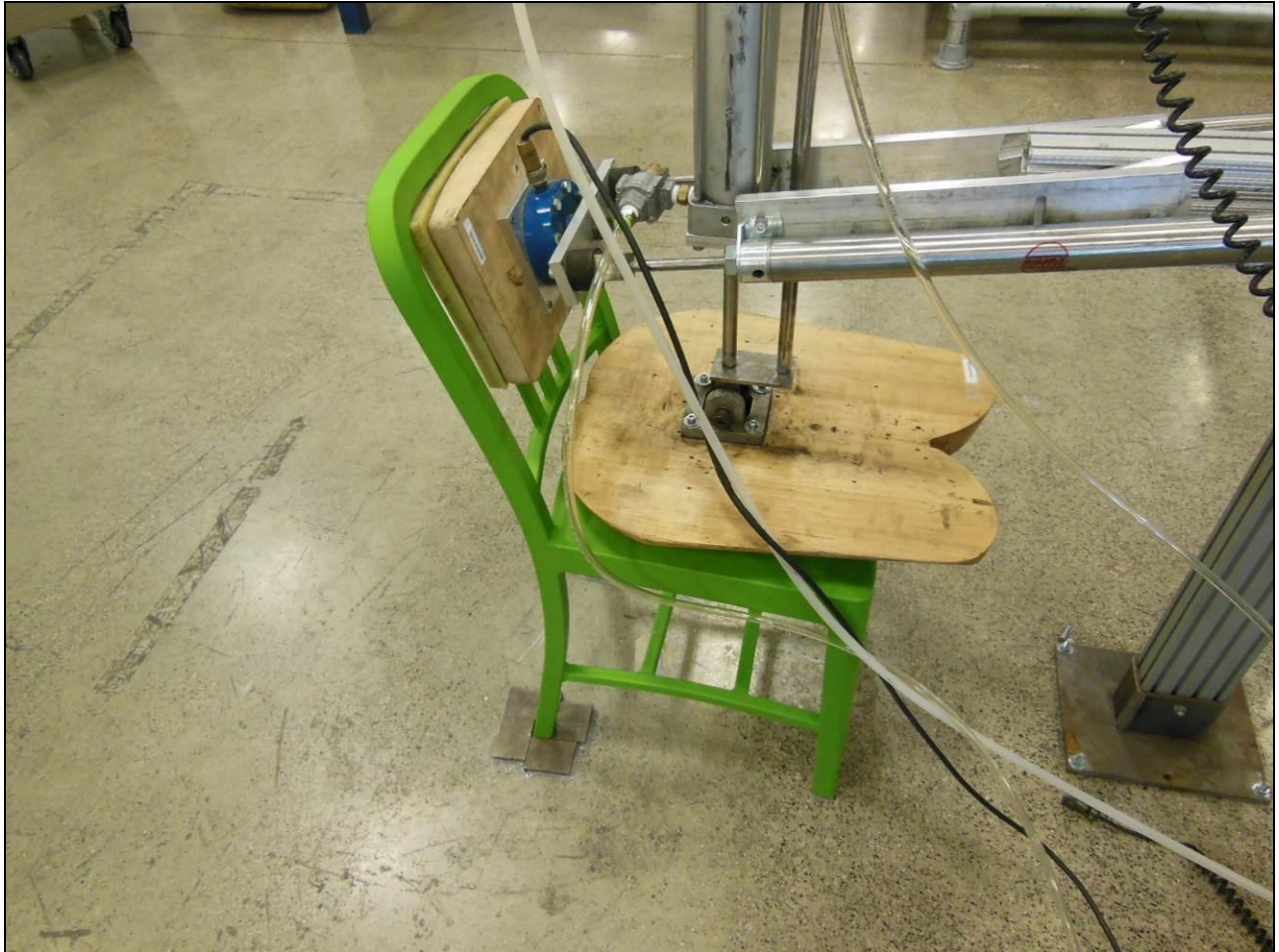
Seat and Back Static Load
