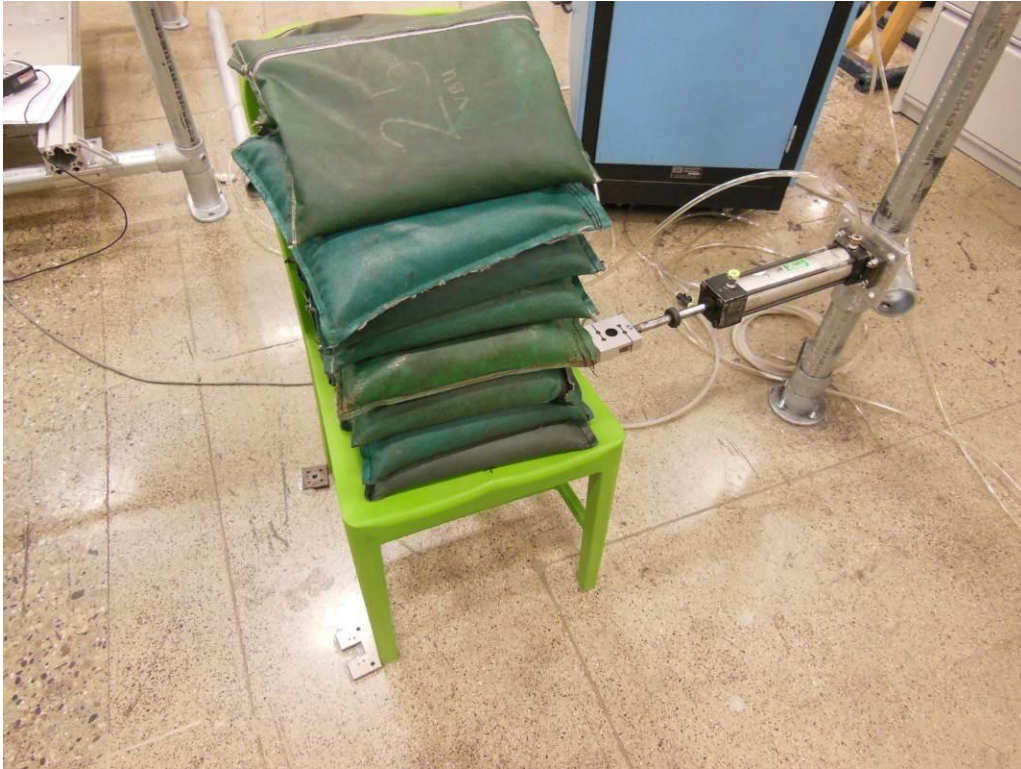
Leg Sideways Static Load
