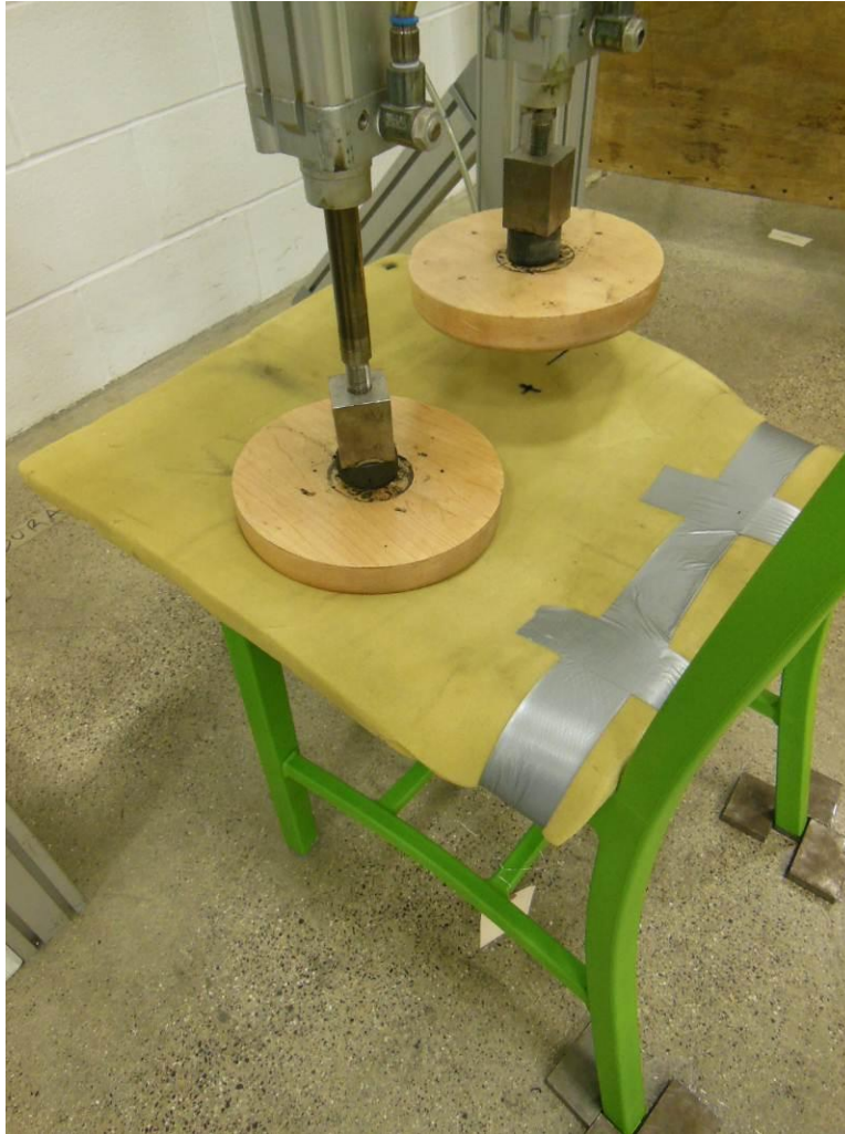
Seat Front Edge Durability
