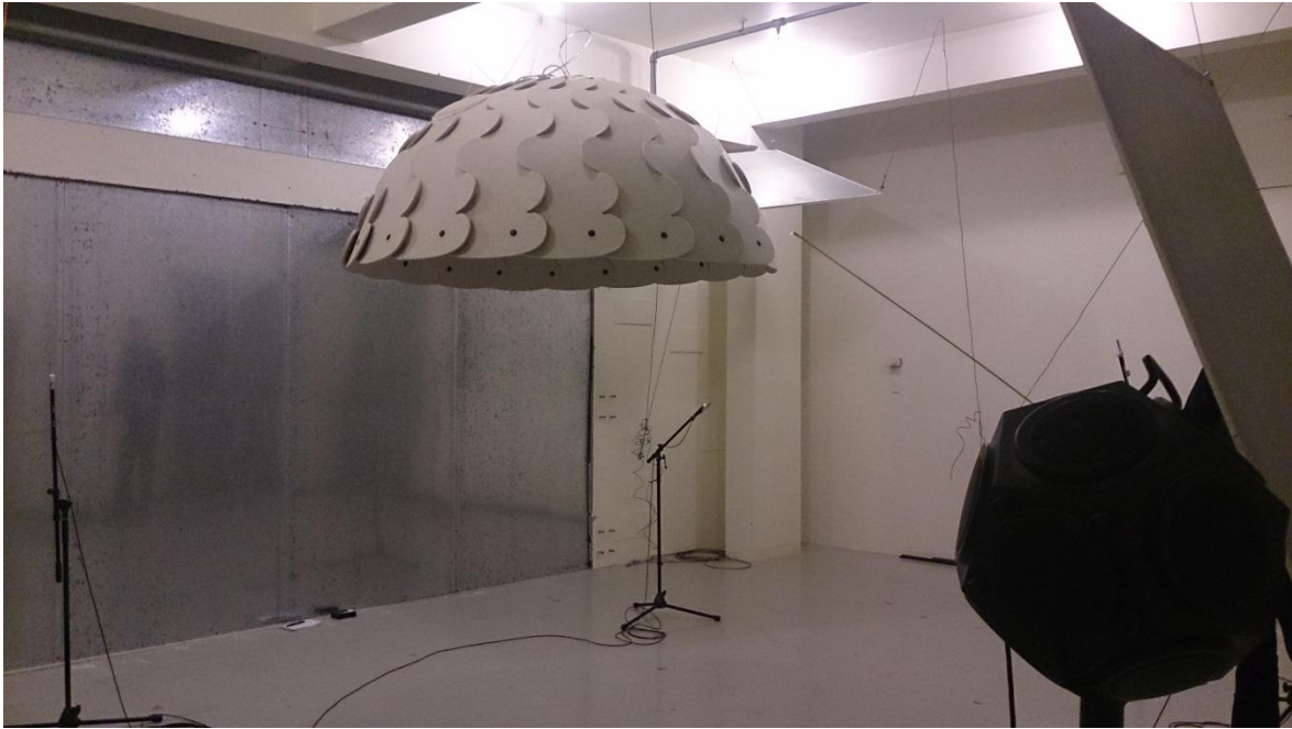
Figure 5: Hush Light Round installed in the reverberation room
