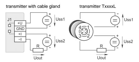
Loop resistance value Rc = R + resistance of wires shall fulfill the condition  $Rc[\Omega] < 40 \times Uss2[V] - 360$ .
