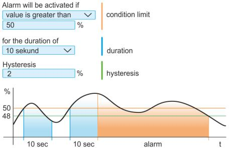
momentary overshoots of the limit value. The hysteresis, too, has a similar significance (*Alarm hysteresis*). It prevents the alarm from oscillating in the case that the measurement value varies around the alarm limit value. It is not recommended to set it equal zero.
