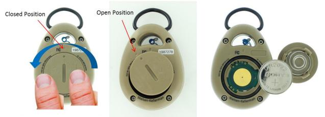
Figure 2: Battery Replacement
