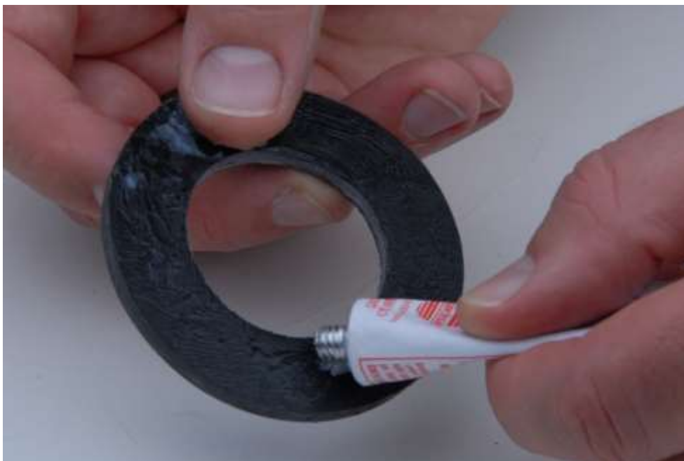
COAT BOTH SIDES OF THE RUBBER WASHER WITH SILICONE GREASE
