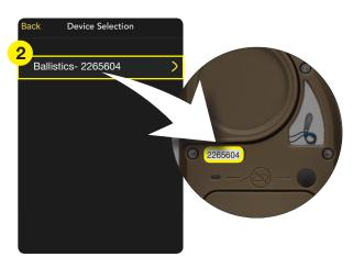
**Trouble Shooting:** Make sure Bluetooth is turned on in your mobile device. Make sure Bluetooth is turned on in your Kestrel and set Connect to PC/Mobile in the Bluetooth Sub Menu. Your Kestrel will not appear on the Bluetooth connection menu in your mobile device. Use the Device Selection button in the app to connect.
