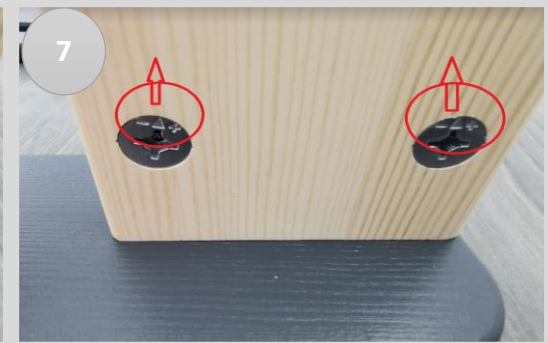
7 Tighten the lock clock-wise till the arrow will point opposite direction of the bolt. Do not overtighten or the lock can be damaged! Do it for all of the locks on both sides.
