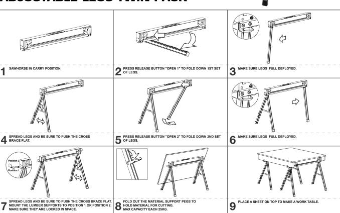
**WARNING!** TO REDUCE THE RISK OF PERSONAL INJURY, READ AND UNDERSTAND THE INSTRUCTIONS. SAWHORSE LEGS MUST BE FULLY OPEN WITH CROSS BRACE LOCKED DOWN. DO NOT STAND ON SAWHORSE. DO NOT OVERLOAD. MAXIMUM CAPACITY 500 KG. USE ONLY ON A FLAT, DRY, HARD AND LEVEL SURFACE.
