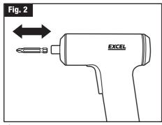
MARNING: Check that the accessories are correctly attached. Incorrect or insecurely fastened accessories can come loose during operation and cause a hazard.
