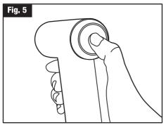
Your tool is equipped with a Forward, Reverse rotation control (6). It was designed for changing rotation of the chuck. Touch the Forward, Reverse rotation control (6) to exchange the screwdriver forward and reverse. The green light of the forward and reverse rotation indicator ring (4) indicates the forward status. The red light of the forward and reverse rotation indicator ring (4) indicates the reverse status.
