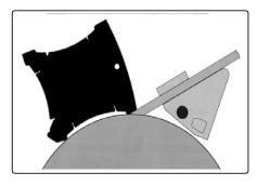
Remove angle measurer from wheel, lift edge of tool from wheel, ensure nothing is in contact with wheel.Start Wheel by using on/off switch.
