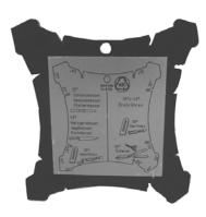
Place Angle measuer on wheel to obtain correct sharpening angle, adjustment canbe made by adjusting tool rest support.
