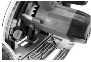
2.Press the Knob inwards and slide to set the desired depth using the Cutting Depth Scale.
