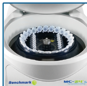
Unique Combi-Rotor™ Accepts tubes and strips
