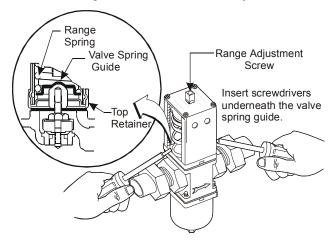
Figure 2: Manual Flushing V46\_union\_flush.cdr
