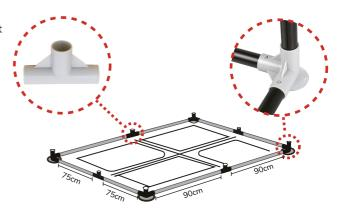
Insert the vertical tubes into the play pen cover and insert the T-shaped tee and the sucker tee to complete the joining of the middle of the play pen wall.
