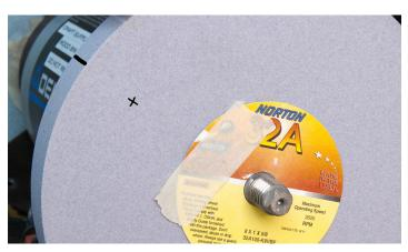
**4.** Place a single layer of tape on the paper washer on left side of the wheel with the tape positioned opposite the tape on the right side paper washer. Example: If the tape on the right side of the wheel is at 10 o'clock, the tape on the left side of the wheel should be located in the 8 o'clock position. If done properly, the tape on opposite sides of the wheel are positioned 180 degrees from one another.
