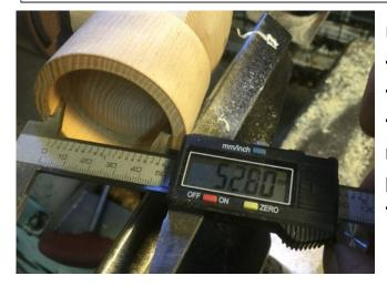
Use a set of vernier to measure the tips of the female threads. Wobble the verniers slightly when touching the threads to ensure you have maximum diameter but not so much pressure that you damage the threads. On the sample it is 52.8mm
