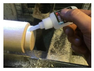
Run some thin Cryo glue on the part to be threaded. Wipe / spread with tissue then activate the glue.
