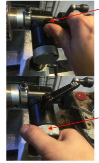
Click the front silver knurled dial anti clockwise about 3-4 clicks so the cutter is free from the wood. Turn the cutter by hand first to ensure its not touching the work. Then turn on the lathe and run the cutter at approx 3000 RPM
