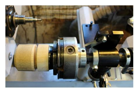
Now lift back again using the hinge plate to check your thread. If you have made the spigot 100% the correct size the threads should work. But don't worry if the threads are still tight. If they are follow the next steps on page 8
