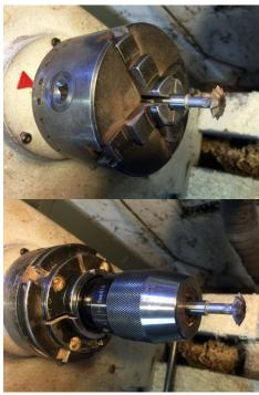
Engineering jaws on an axminster or similar chuck. Best method when holding the cutter as far out as safely possible allowing long threads to be cut when making wooden threaded rings.
