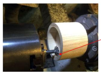
Then with the cutter touching the wood, pivot the work until you can see the chuck is
