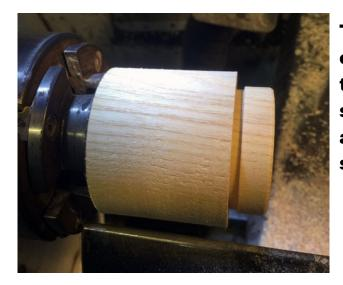
Turn the male spigot to exactly the correct size. This will ensure that the thread will fit first time. Make a shoulder relief cut about 3mm wide and deep so the thread cuts into this space.
