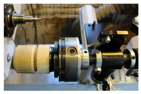
Now you can use the hinge plate to check. Ensure the cutter is clear, undo the front lever and lift the jig and chuck towards you. This will allow you to check the fit. It should still be tight but sometimes the box may fit at this stage. Its good to check.
