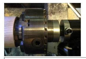
Keep the work in the chuck and unscrew the chuck from the lathe and thread onto the threading jig.
