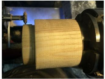
Now move the jig one click at a time with the cutter spinning in the lathe until you have the cutter just starts touching the wood. You can hear when this happens. This is now zero.
