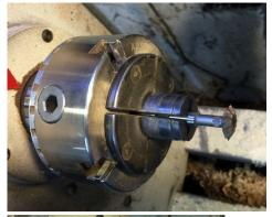
Using pin jaws on another chuck works fine.
