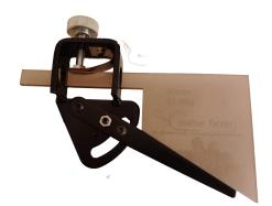
Two sets of templates have been developed which can be used to consistently set the angles accurately.
