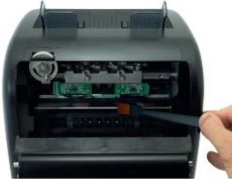
1. Open the Upper back cover using the handle and place the white plastic strip in the machine. Please clear the sensors prior to performing this task using the brush provided as part of the maintenance kit
