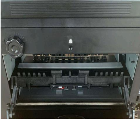
1. Open the Upper back cover using the handle, place the white plastic strip in the machine and close the back cover
