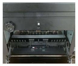
Open the Upper back cover using the handle, place the white plastic strip in the machine and close the back cover
