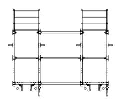
Note: X-Racks are required to be bolted to a concrete sub-floor
