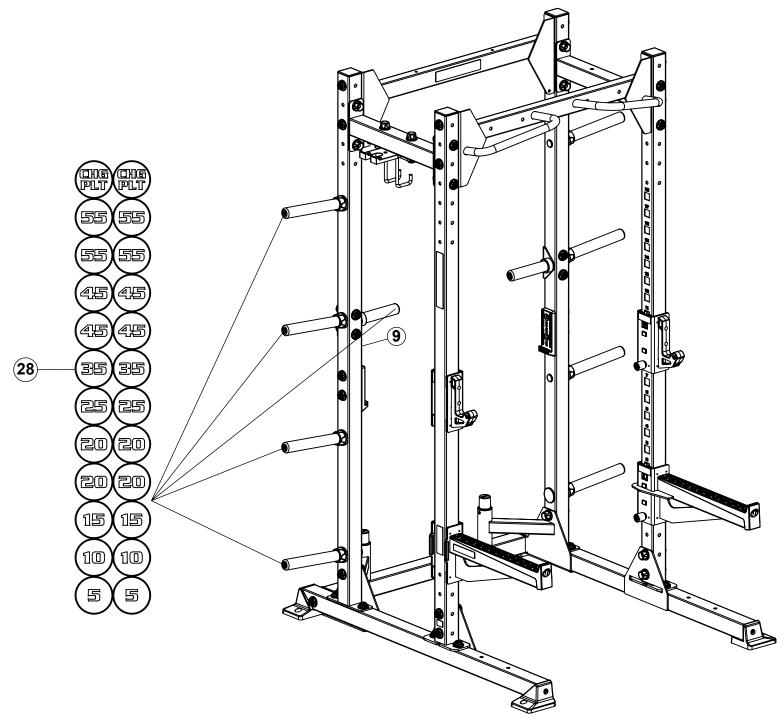
Using a rubber mallet, install the desired WEIGHT STORAGE NUMBER CAP into the end of the WEIGHT HORN.
