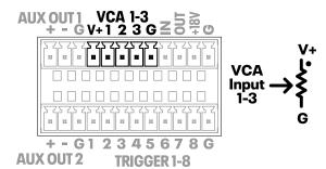
Remote DC level control is available on these three VCA (voltage controlled amplifier) inputs. A VCA Gain block is first placed in any input or output signal chain, then assigned to a VCA input. Multiple VCA gain blocks can be assigned to the same VCA input pin.
