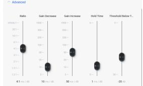
**Threshold Below Target** - Determines the relative input signal level above which the autoleveler increases gain, below which no action is taken.
