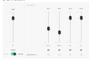
A DCA gain block can be placed on any channel in order to assign that channel to DCA groups 1-4. The channel's overall level to all DCA groups, plus the level to each of the four DCA groups is individually adjustable.
