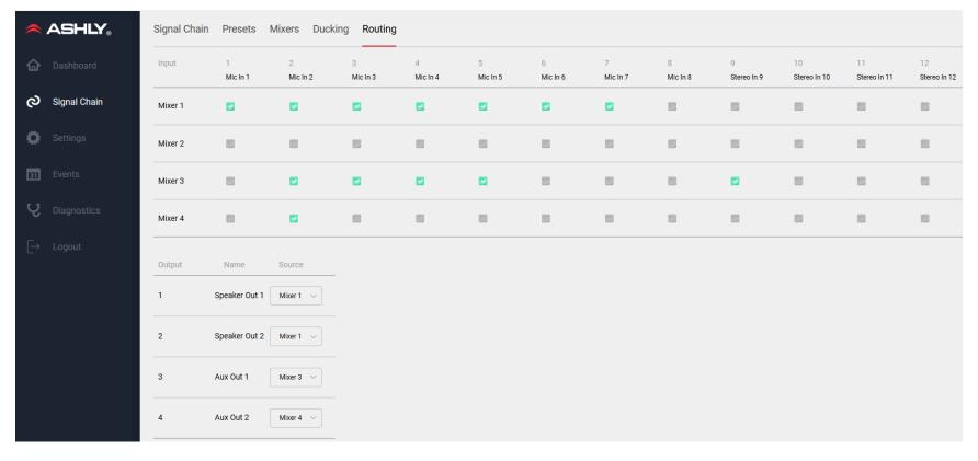
The signal chain routing screen allows fast setup and review of all input and mixer signal routings, plus mixer source assignment for the two amplifier channels and two aux outputs.
