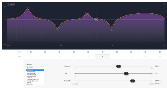
The PEQ parametric equalizer provides a variety of powerful filters for adjusting signal response with precision. A master on/off button enables/disables the PEQ block.
