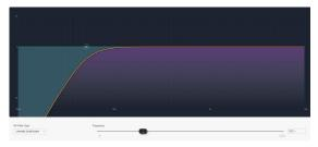
A high-pass filter (HPF) is a single ended filter without a level control, passing only signal above the selected corner frequency. Filter types include Bessel, Butterworth, Linkwitz, and Linkwitz Notch, including a variety of filter slopes.
