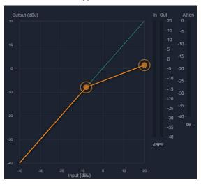
An attenuation bus assignment is provided to allow multiple limiters to force their gain reductions to track each other, ie for stereo signals. For peak limiting with infinite ratio, use the brick wall limiter function.
