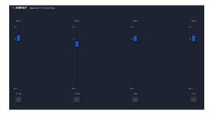
DCA groups are used to globally adjust the relative levels of all channels assigned to that group. In the DSP signal chain, a <u>DCA block</u> must first be placed on every channel you wish to assign to a DCA group, then enabled and adjusted for each DCA group as desired. A remote operator profile can be created granting limited permission to use Remote DCA on a tablet or mobile device.
