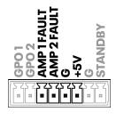
into protect mode, the amp fault output pin for that channel goes logic low.
