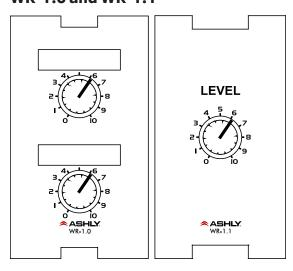
The WR-1 and WR-1.1 are remote level controllers used for DC level control inputs.
