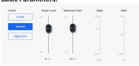
**Target Level** - The desired continuous output level of the signal.
