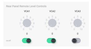
The three back-panel VCA (voltage controlled amplifier) input pins are used to remotely control the level of assigned inputs or outputs using a simple potentiometer circuit.
