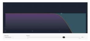
A low-pass filter (LPF) is a single ended filter without a level control, passing only signal below the selected corner frequency. Filter types include Bessel, Butterworth, Linkwitz, and Linkwitz Notch, including a variety of filter slopes.
