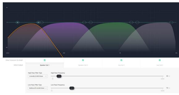
Crossover blocks can be placed on both speaker and Aux output channels. A high-pass and low-pass frequency is applied for each crossover filter, along with filter type, to bandlimit the signal for that output.
