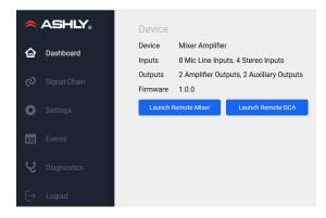
The dashboard is the software screen where the mXa-1502 first appears after logging in with your browser. The dashboard shows the Ashly device, number of inputs and outputs, and firmware revision.
