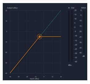
The brick wall limiter is a compressor with a fixed infinite ratio. Use a brick wall limiter to prevent signal from exceeding a designated peak level. The limiter function allows for threshold, attack time and release time adjustments.
