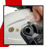
1. TAKE A 1/8" ALLEN WRENCH TO THE SECOND SCREW AND UNSCREW COUNTER CLOCKWISE
