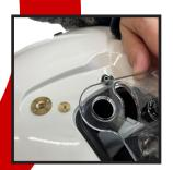
1. TAKE A 1/8" ALLEN WRENCH TO THE SECOND SCREW AND UNSCREW COUNTER CLOCKWISE
