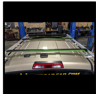
Ensure that your rack is squarley placed on your vehicle, then mark down the location of each slot on the vehicle to drill
