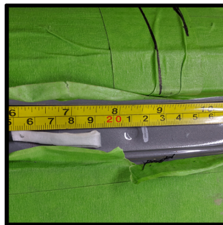
Mark at 8.5" on both the passenger and driver side, these will serve as your guide hole locations
