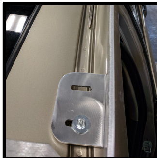
Place the roof rack on the vehicle w/out the spacers and lightly bolt it to the first two installed plusnuts
