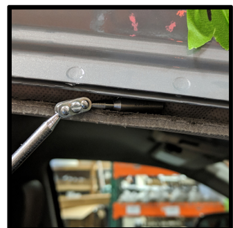
Ensure that your rack is squarley placed on your vehicle, then mark down the location of each slot on the vehicle to drill
