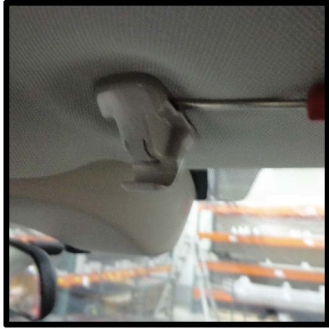
Remove visor clip with small flat head into the opening and pull down clip.
