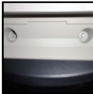
Remove two screws on the sunglasses holder. Pry down to remove assembly.
