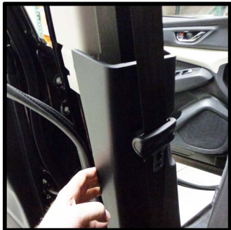
Pull out on the lower B-pillar panel.
