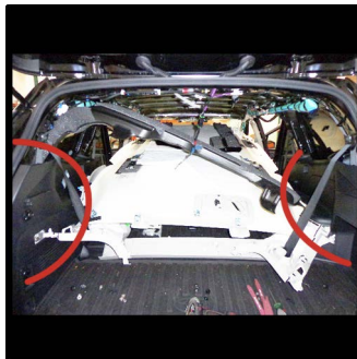
Pull out on lower D-pillar panels. This exposes a clip that will allow the C-pillar panel to be fully removed.
