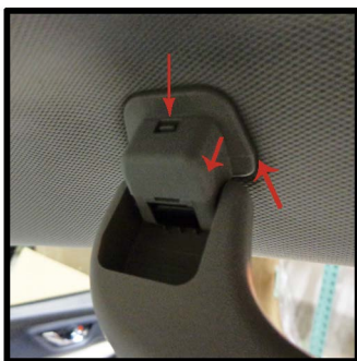
Pull down on tab and out on clip.
