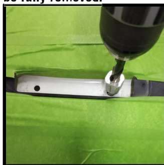
Now with the stock rails removed drill out the holes to 3/8". * Using a drill stop is recommended.
