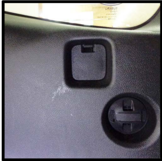
Remove cover to expose screw.
