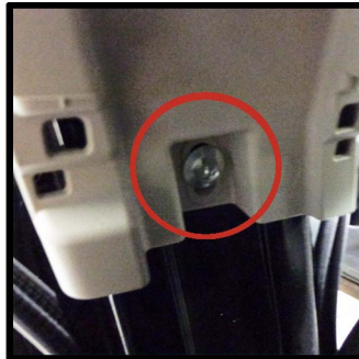
With the lower B-pillar panel pulled back remove the bolt from the upper B-pillar panel.
