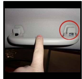
Pull handle down and locate release tabs.
