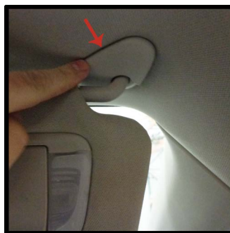
Pull down visor and remove plastic cover.
