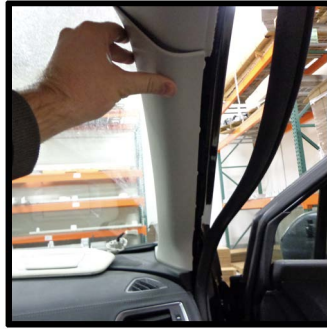
Pull out A-pillar panel.
