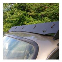
Place the rack on the roof of the vehicles carefully to make sure that the wind deflector is not resting on the roof of the truck. Move the rack forward or back until proper fit is acheived and the maximum surface contact between the raing gutters and the side rails of the rack is acheived.
