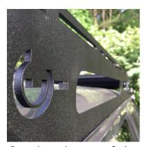
Once the rack is sitting flush inside the rain gutters you can move collect the clamps from your hardare kit and prepare to attach them to the L brackets on your rack and the rain gutter of your vehicle.
