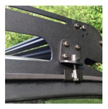
Make sure the rack is centered and loosely secured at all mounting points. Once the rack is in the desired location. Tighten each bolt till the clamp is securely fastened and the rack is secure.
