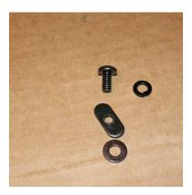
Locate the correct hardware bag containing (10) tnuts, lock washers, flat washers, and phillips machine screws.
