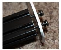
Start by connecting the crossbars to the side rails. You will use (4) 1/4"-20 x1" machine screw, (4) 1/4" flat washer, and (4) 1/4" flat washer per crossbar. Tighten all crossbars loosely as shown in the picture and then go around and tighten them in even increments.
