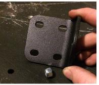
Once the 8 crossbars are connected to the side rails and are all evenly tightened and secure you can then attach the L brackets to the side rails. The L brackets are attached using (4) 1/4"-2- x 1" machine screws, (8) 1/4" flat washers, and (4) 1/4" nylock nuts per bracket.
