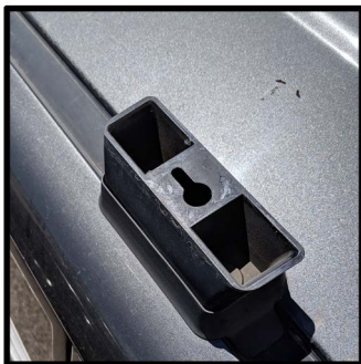
LIFT THE RAILS AWAY TO ACCESS THE LAST TWO BOLTS HOLDING THE CENTER POST TO THE VEHICLE
