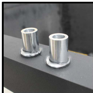
Next place the spacers on the roof
