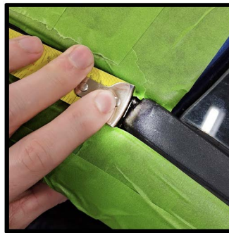
Next place your tape measure up against the edge of the wind shield trim as shown above
