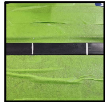
Measure straight back along the gutter trim and mark off at 9\frac{1}{16} ". Then again 4\frac{1}{8} " back from that point. Do this on both the driver and passenger side
