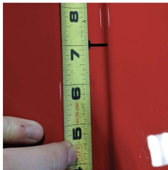
Mark off at 7 inches on the driver and passenger sides. These will act as your guide holes later in the process
