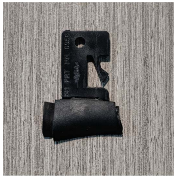
The weather stripping is held in place near the windshield by the clips shown above. Press in the tab to remove
