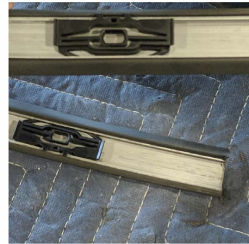
The remaining attached portion can be removed by sliding the strip backwards and then lifting up to release the clips shown above
