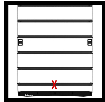
Now attach the crossbars. Except the furthest forward which will be attached later. Make any adjustments if needed to make sure the rack is square then fully tighten it down.
