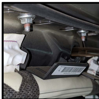
To remove the stock roof rails there are seven nuts that need removed
