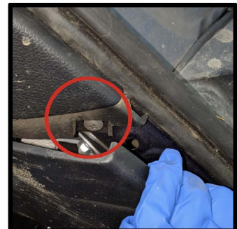
This allows you to pull the panel back to expose a screw holding the upper panel in place
