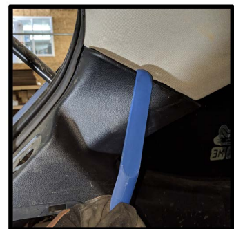
Using a plastic removal tool begin removing the panel around the lift gate supports
