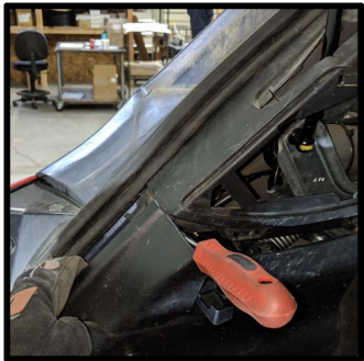
The bottom of the lift gate support panel is covered by a panel below which must be pryed back
