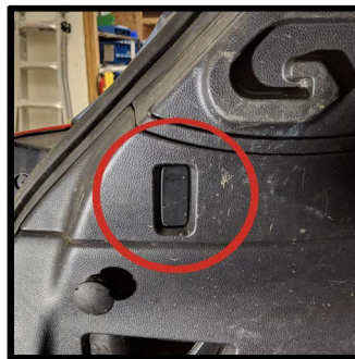
Beginning in the rear of the vehicle there is screw behind the circled tab that needs removed
