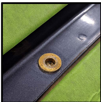
Fully installed plusnut
