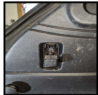
Push the tab down to expose the screw and remove
