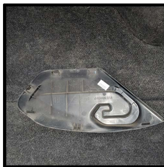
It's attached by plastic tabs around its perimeter
