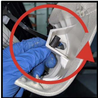
To fully remove the A pillar panel you must rotate the retention hook to slide it out
