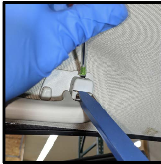
Use a flat head screw driver to depress the release tab then pull up and out
