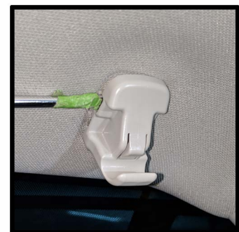
To remove the sun visors first remove the hanger tab
