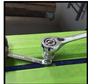
Compress the plusnut by using a 1/2" wrench to hold the coupler & tighten with an 11mm wrench
