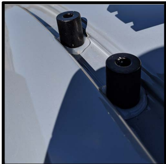
Apply more silicone over the plusnuts before placing the spacers down to ensure a water tight seal
