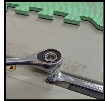
Compress the plusnut by using a 1/2" wrench to hold the coupler and tighten with a 7/16" wrench
