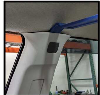
Now pull back out on the top and sides of the upper B-Pillar trim to remove
