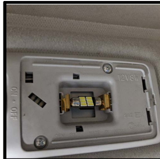
Remove using a phillips head screw driver
