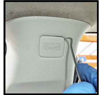
Then remove the plastic cover piece shown above from the B- pillars
