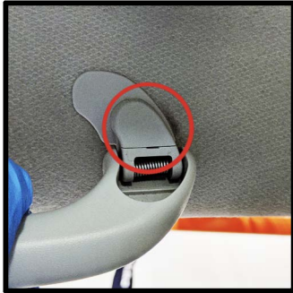
To remove the assist handles from the front & rear remove the covers w/ a flathead
