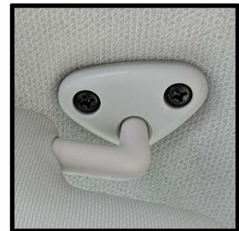
Remove the visors on each side by taking out the philips head screws ...
