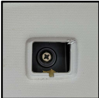
Remove the screw using a 10mm socket
