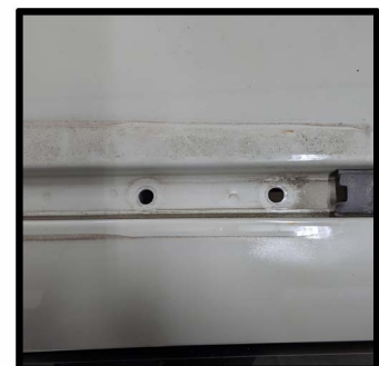
It may be necessary to clean up the holes with a 3/8" drill bit to allow the plusnuts to fit
