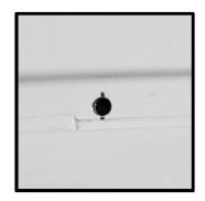
Next drill in the center of your channel a 3/8" hole on both sides at the 10" mark. These will act as guide holes later in the process
