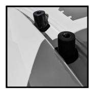
Then place the spacers down with a liberal amount of silcon before placing the rack back on the roof
