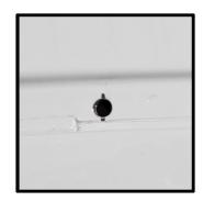
Remove the roof rack and drill out he remaining holes
