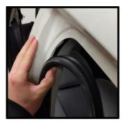
The rubber trim around the doors can be pulled back to collect any metal shavings that have fallen to the headliner
