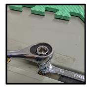
Compress the plusnut by using a 1/2" wrench to hold the coupler and tighthen with a 7/16" wrench
