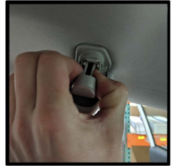
Pull each side of the handles out.
