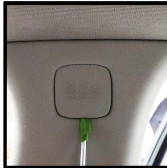
Now begin removing the B-pillar trim.
