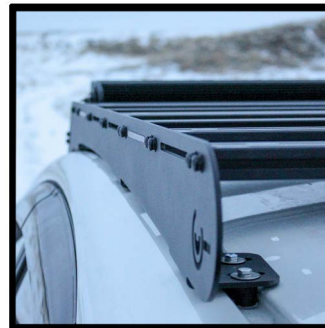
Apply more silicone and place the spacer on the roof.
