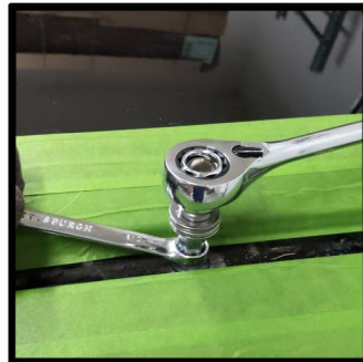
Compress the plusnut by using a 1/2" wrench to hold the coupler & tighten with an 11mm wrench.
