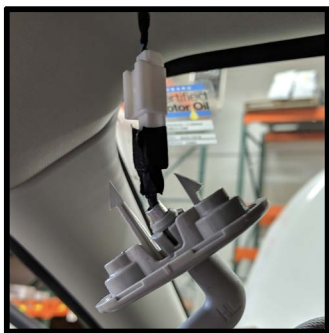
Next disconnect the white plug that powers the mirror lights in the visor.
