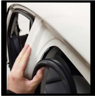
Remove the rubber trim along all of the doors.
