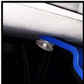
The paneling by the rear seat is held in by several plastic clips.
