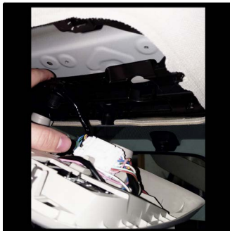
Dome panel can now be pulled down and unplugged.
