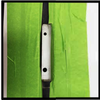
View of bottom hole drilled, be sure to clean any shavings away that fell thru while drilling.
