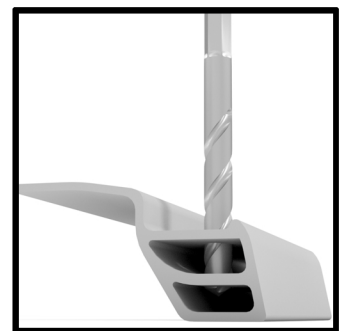
The rest of the mounting holes will require drilling thru both channel layers as shown above to a diameter of 25/64"
