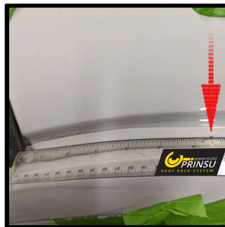
Measure back 6-1/2" from the top corner of the windshield and mark with a punch
