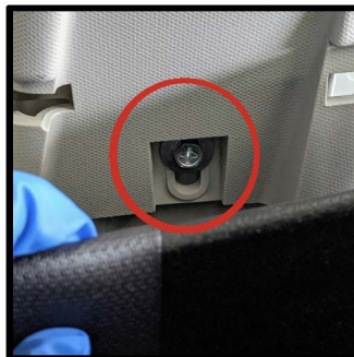
Remove using a 10mm socket
