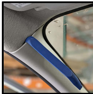
Disconnect the A - Pillar trim by first pulling out from the top
