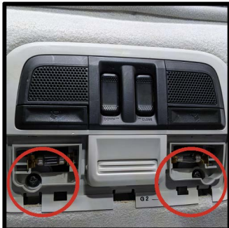
Remove the two circled screws
