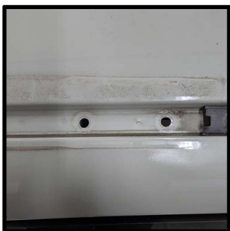
It may be necessary to clean up the holes with a 3/8" drill bit to allow the plusnuts to fit
