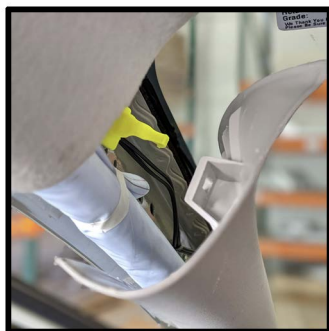
Retention hook rotated and trim fully removed
