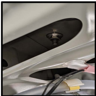
The far rear nut can be reached via the access holes in the vehicle structure shown above
