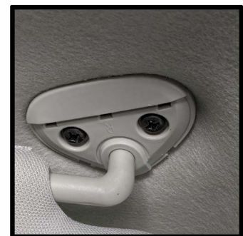
Remove the screws with a phillips head screw driver
