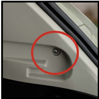
In the rear remove the screw circled above on both sides
