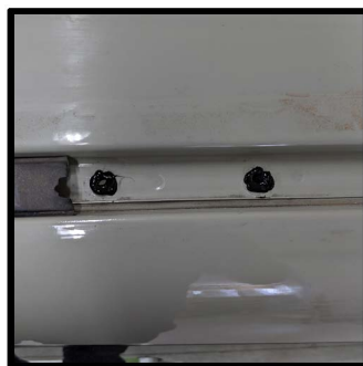
Before installing the plusnuts apply a small amount of silicon around the holes
