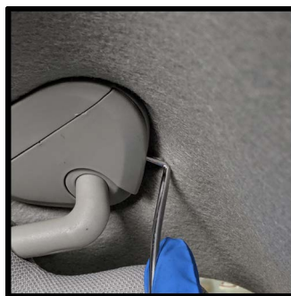
Next remove the sun visors by first popping off the plastic covers to expose the screws
