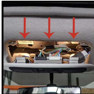
Grab along the edges and carefully pull down
