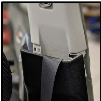
Pull the lower portion of the B-Pillar trim back to expose the remaining screw
