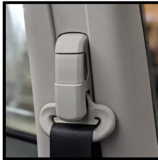
Remove plastic cover to access seat belt bolt
