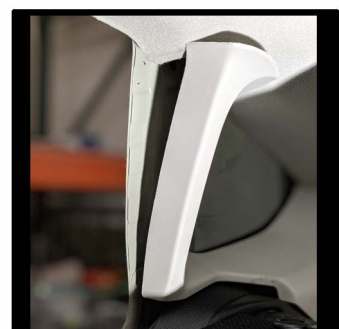
Remove the rear seat passenger assist handles then move to the C-Pillar trim to remove
