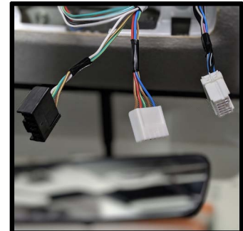
Disconnect the plugs running to the dome light and control panel unit
