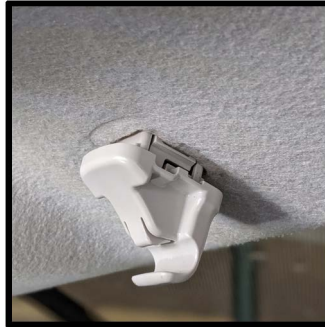
Hanger released and partially removed
