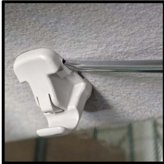
To remove the visor hangers use a flat head screw driver on both sides to release the internal plastic tabs
