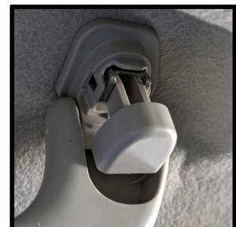
Retainer pulled out, the assist handles can now be fully removed
