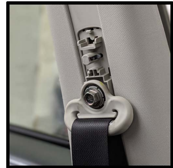
Remove using a 15 mm wrench. *When reinstalling torque to 22.1 ft-lbs*
