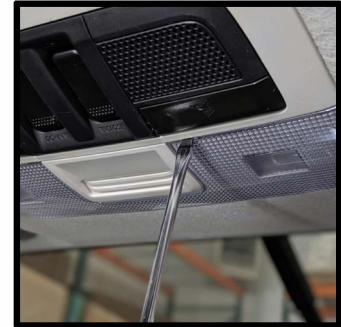
To remove the over head dome light and control panel pop the light cover off
