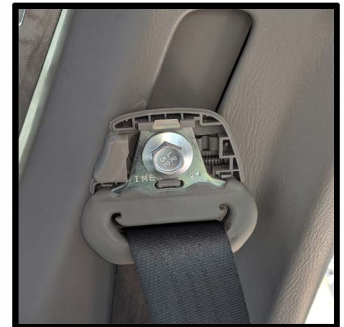
Remove the 15mm bolt, then the seat belt and trim behind
