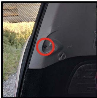
Remove the screws circled above in this step and the following three steps
