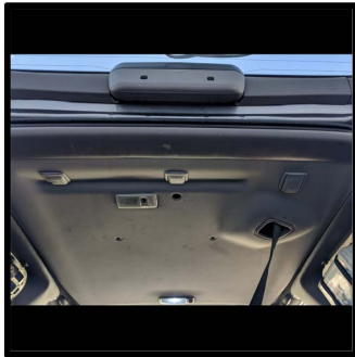
Begin the headliner removal in the rear of the car
