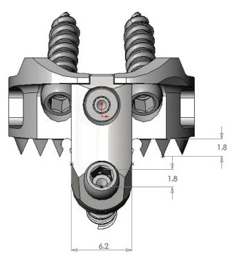
Fig. 3 8x15mm InterPlate™ Assembly
