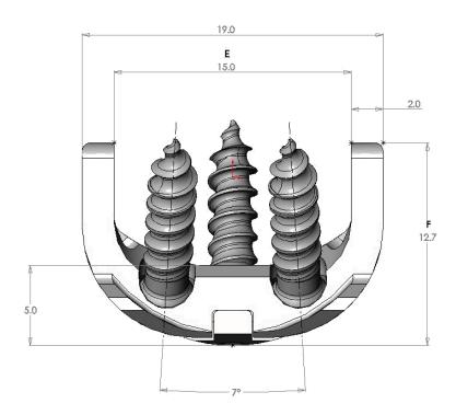
Fig. 2 8x15mm InterPlate™ Assembly
