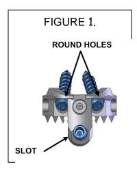
as subsidence occurs. The length of the slot is matched to the height of the teeth so that when the teeth are fully embedded the screw is at the end of the slot.
