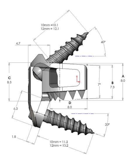
Fig. 1 8x15mm InterPlate™ Assembly
