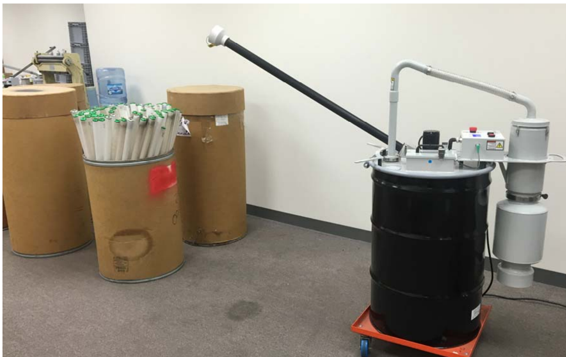
Figure 3 Bulb Eater® 3L in Office Area – Test 2
