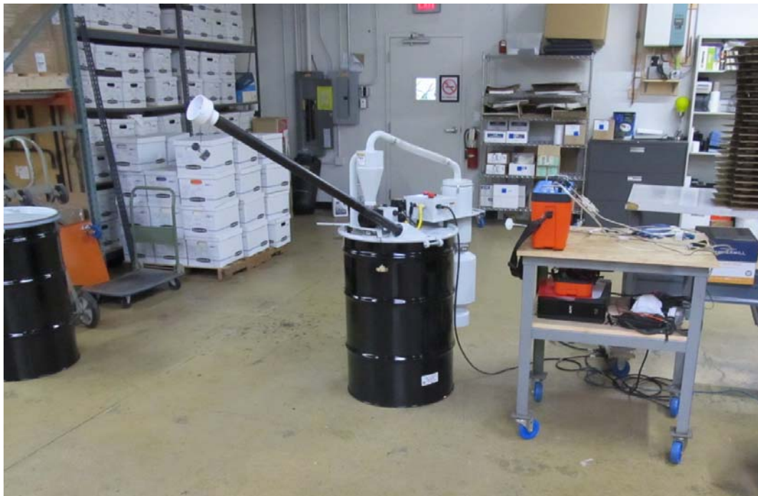
Figure 2 Bulb Eater® 3L in Warehouse Area – Test 1
