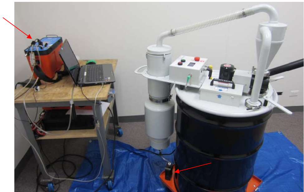
Bulb Eater® 3L testing set-up showing portable battery-powered sampling pump and Mercury Tracker 3000 IP
