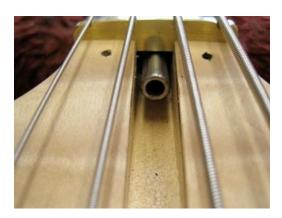
In this position the Truss Rod works in exactly the opposite way as a traditional Truss Rod does. Turning the nut clockwise will again tighten the Truss Rod, but in this position, it will <u>increase relief / bow in the neck</u> and move the strings away from the fingerboard. Turning the Truss Rod Nut counter-clockwise will loosen the Truss Rod and decrease relief / bow in the neck.
