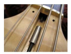
2. Now thread the Truss Rod Remover into the threaded portion at the top of the Truss Rod. You only need to thread the tool 2-3 complete turns.
