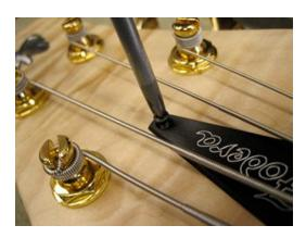
3. Remove the Truss Rod Cover. <u>In order to ensure the proper adjustment of your Truss</u>
