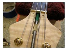
6. Insert the Truss Rod to approximately this depth.
