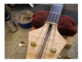
3. Pull the Truss Rod of the channel in the neck.
