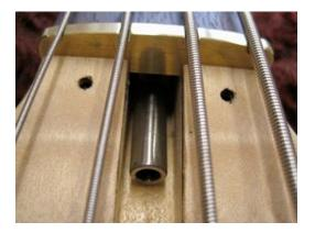
In this position the Truss Rod works in the same way that most typical truss rods do – <u>turning the nut clockwise will tighten the Truss Rod and decrease relief / bow in the neck</u> thereby moving the strings closer to the fingerboard. <u>Turning the nut counter-clockwise will loosen the Truss Rod and allow the tension of the strings to increase relief / bow in the neck and serve to move the strings further away from the fingerboard.</u>
