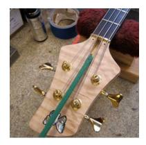
4. Whichever position the Truss Rod was in, flip it over 180 degrees before reinserting it into your bass. In the photos that follow, a Truss Rod that had been in the Normal Position is being flipped to the Reversed Position.
